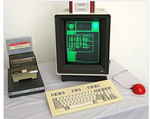
DMD 5620 terminal, based on the Blit , connected to a SVR3 host and showing the Layers interface
